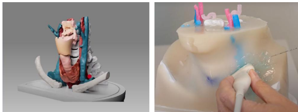
Figure 2 The ad-hoc 3D model designed for operators' training. This model consists of 3D printed anatomical structures (on the left) plunged in an agar-based gel (on the right) which produces the same echogenicity as the human body
